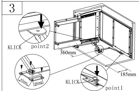
C. Adjusting location of wag frame well. first fixed two side of it on the two frames, then fixed fame base in frame according to the location wiht screw.
