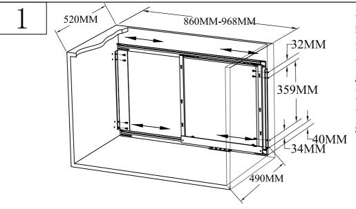
A. Fixing the main slide-out frame in frame with screw accordind to location size as the picture show.
