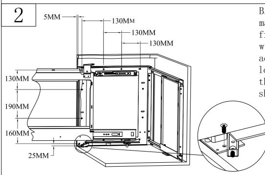
B. Fixing the main inclined frame in frame with screw according to location size as the picture show.
